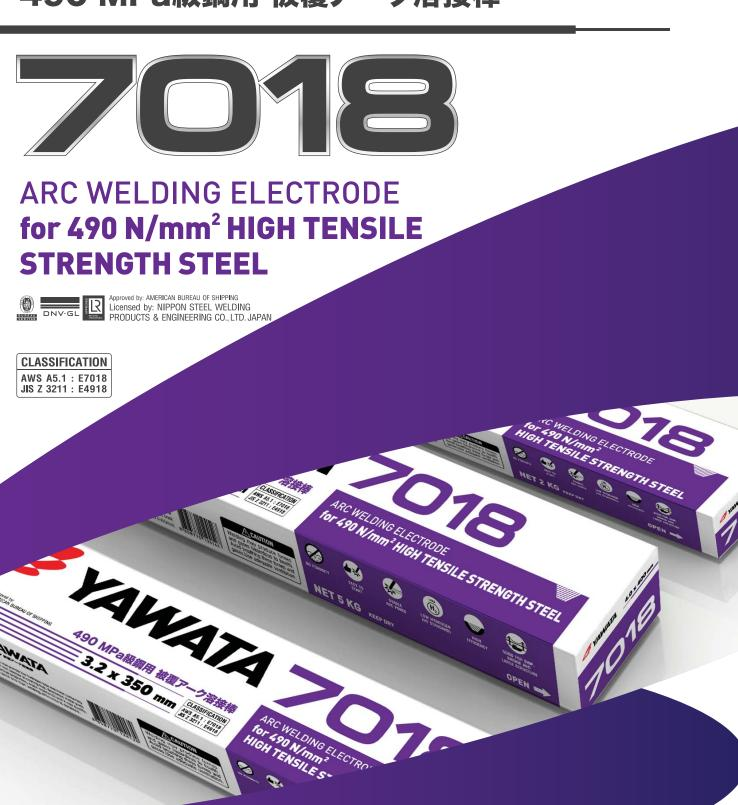
YAWATA 7018 is an iron powder low hydrogen type electrode containing a large amount of iron powder in coating flux. Deposited metal gives excellent mechanical properties, crack resistance and X-ray quality. Weldability is good and high welding efficiency is obtained.
